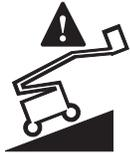
Light on indicates the machine is not level. The tilt alarm will be sounding when this light is on. Move the machine to a firm level surface.
